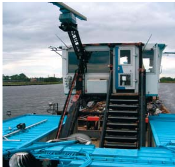
Fig. 3. The superstructure of ODRA LOYD 9 ship
